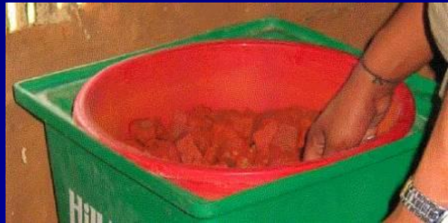
Placing brick chips in the diffuser box
