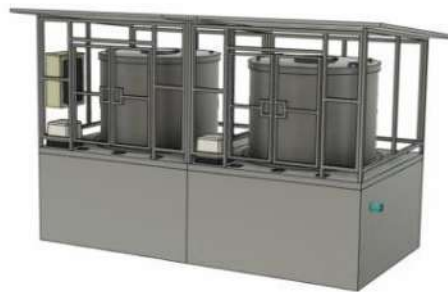
2 x Aquonic 1000 with 8000L Septic Tank & Solar PV Energy System
